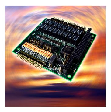
High-Density 32-Channel PC/104 Board Provides Change-of-State Detection, Optically Isolated Digital Inputs, Relay Outputs and Low Cost (104-IIRO-16)
