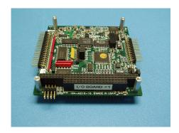
Note: Plan your I/O stack so that cable lengths and cable locations on the I/O plate and board itself are taken into consideration for painless assembly.
