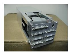
Note: When installing I/O Plate to Bottom End Plate keep in mind to install in such a way which eases the routing of the various I/O cables.
