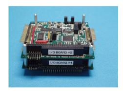
6. Repeat step 4 for each additional I/O BOARD then plug in the CPU on top of the stack. Install 4 x 0.475" M3 m/f standoffs to secure the CPU to the top I/O BOARD along with a small application of loctite to the threads.
