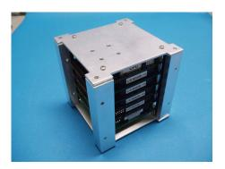
Note: Some separation may be necessary between power supply and I/O BOARD #1. This tolerance is built into the design and allows for fine tune adjustment to ensure proper heatsinking of CPU and power supply.
