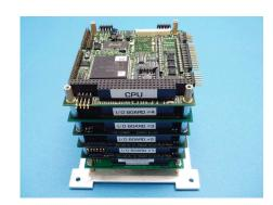
Note: If the CPU you are using has any cable locations which are not available at the boards edge, now would be the time to install these cables.
