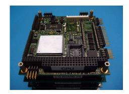
12. Install Top End Plate, with heat sink attached, to the CPU board and secure with 4 x 0.5" M3 screws and a small application of loctite to the threads. Tighten until heatsink makes solid contact with the CPU microprocessor without bending the CPU board.
