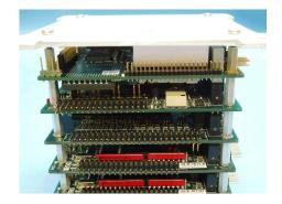
13. Install rails on corners of the stack.
