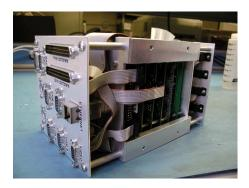
Note: When installing CPU Plate to Top End Plate keep in mind to install in such a way which eases the routing of the various CPU cables.
